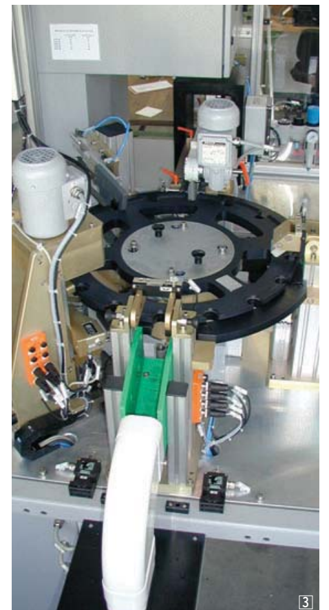
Photo 2+3: Typical system with test stations for crack detection and structure test. An optional master part run will guarantee constant test quality.
